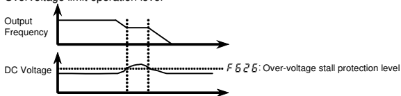
Overvoltage limit operation level
